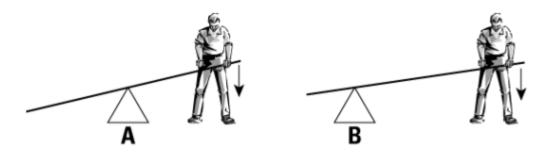
In which of the two figures will the person require less force to lift a 50-pound weight?
